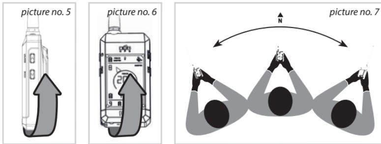
**WARNING:** Accuracy of the direction arrow (pointing to the north) depends on the correct calibration of the electronic compass. Calibrate properly again, when the indication of the direction to the dog is inaccurate.
